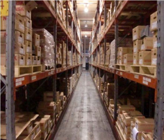
Narrow Aisle Racking
